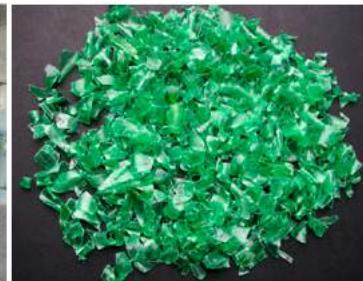
*Compressed plastic waste, plastic flakes from recycled waste – photo credit to “Eco Engineering”.*
